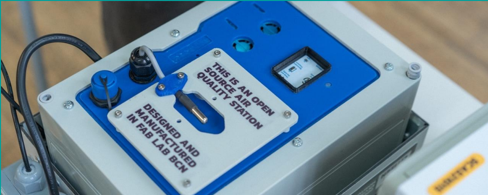
An open-source air quality station designed and manufactured by Fab Lab Barcelona. Image source: Creative Commons
