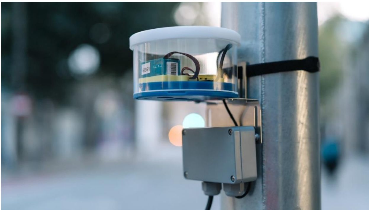
The SCK 2.1 outdoor particulate monitoring device (developed for the Smart Citizen program) deployed on a street pole. Image source: Creative Commons
