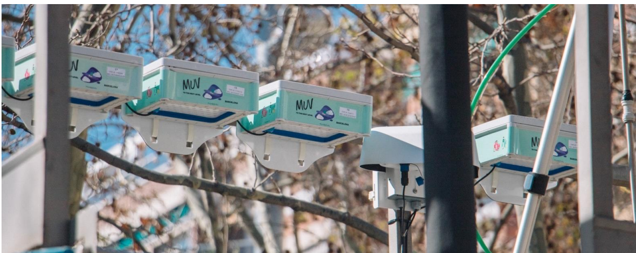
DIY air quality sensing devices created at Fab Lab Barcelona, co-located with a regulatory air quality monitoring station. Image source: Creative Commons
