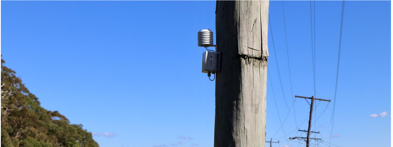
A large, solid street pole can block communications between a device and a nearby gateway. By considering orientation, this problem can be avoided. Image source: Lake Macquarie City Council
