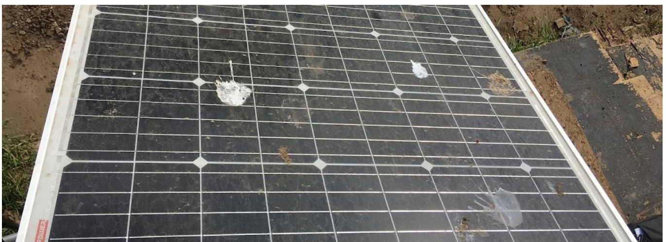
Even mild fouling of a solar panel can be enough to completely impair its function. Image source: UTS.
