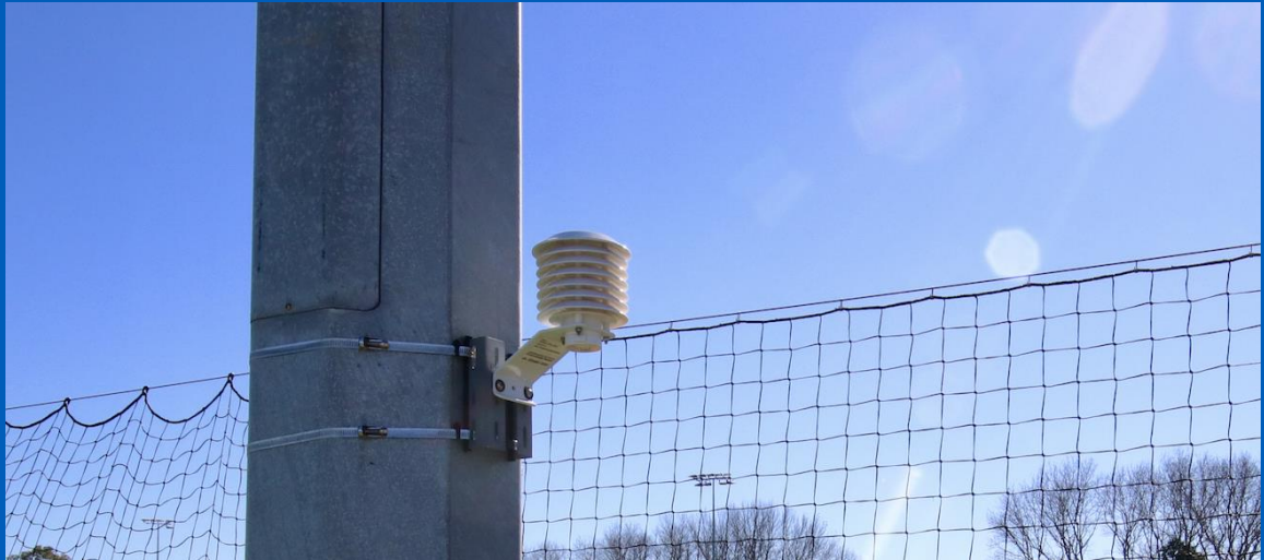
A temperature and humidity monitoring device featuring a Stevenson shield. Image source: UTS
