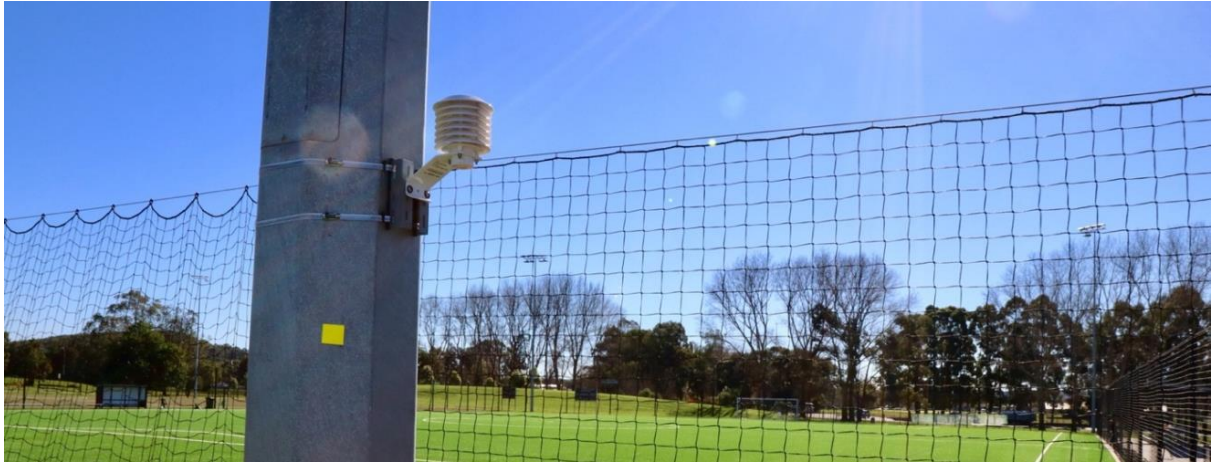
Battery-only power supply is usually limited to small temperature and humidity sensing devices like this one. Almost all air quality sensing devices require solar or mains power. Image source: Lake Macquarie City Council
