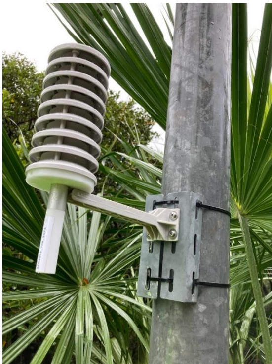
A temperature sensing device fitted with a solar radiation shield. Image source: UTS
